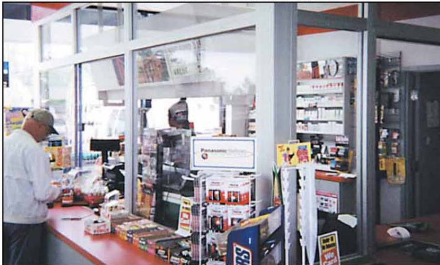
The clerk at this convenience store opens the Bullet Resistant Sliding Window for "business as usual" during the day. At night, the clerk closes the window for maximum protection.
