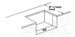
26" OR DEEPER COUNTER BEHIND THE WALL (INCLUDES WALL THICKNESS)
